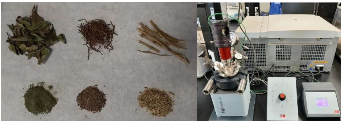
Figure 5. Stevia leaves, roots and stems are pretreated by ultra-high-pressured reactor to produce fructooligosaccharides
