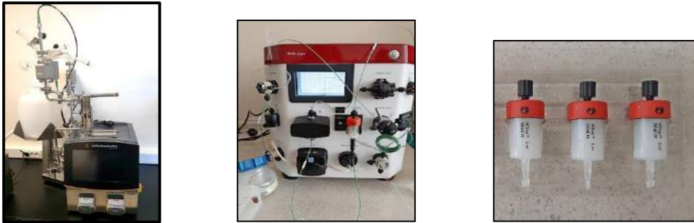
Figure 6. Purification steps of mannanase. Ultrafiltration and chromatographic purification
