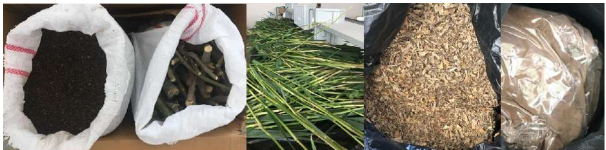
Figure 5. Feedstock (from left to right: olive pomace, olive tree pruning waste, reed, oak tree waste and cork dust)
